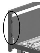
Loosen the screw at the bottom of the C-rail, remove the fitting downwards and replace the screw connection.
