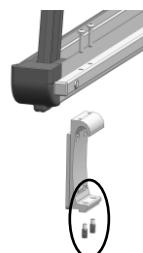
The next step is to mount the holder to the SR1 side rail using the pan-head screws.
