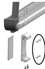
The next step is to lightly screw the threaded rods into the aluminium bracket.
