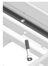
Press the cover plugs into the open holes.
