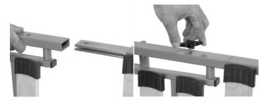
3. Push one end piece on one side completely and screw tight.
