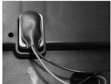
9 V block battery for emergency lowering
